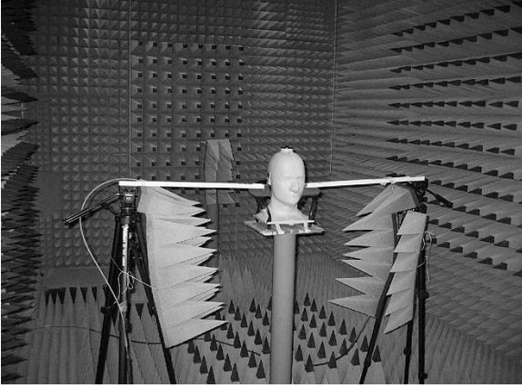
Fig. 1. Measurement setup with SAM head phantom in the anechoic chamber.
